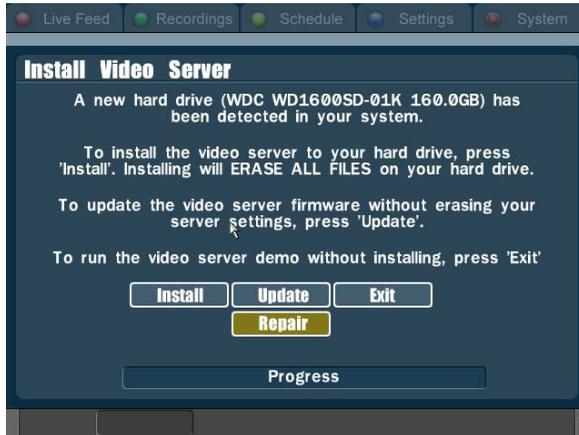
**Figure 61. Tsunami™ Installation Menu**
