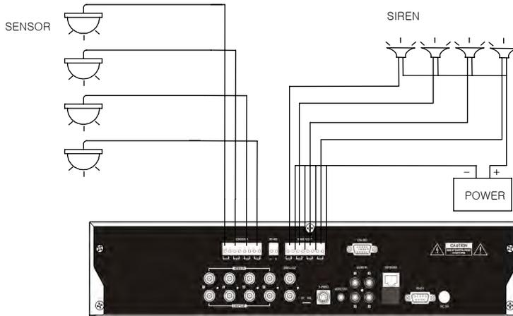
Sensor In : Connect the sensors.
