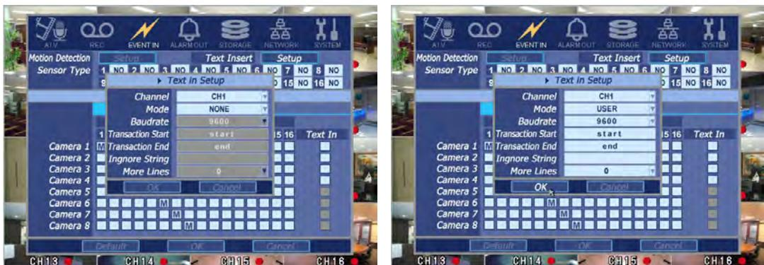
Go to the wanted channel , use the left and right arrow key to select the device. If you cannot find your device, please contact our technical support. The advanced setup of the device will be performed by client software.
